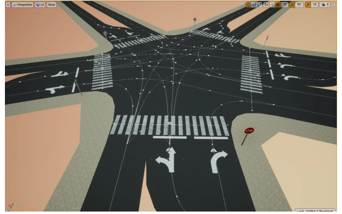
Fig. 4: A five-way intersection generated using IntGen.
